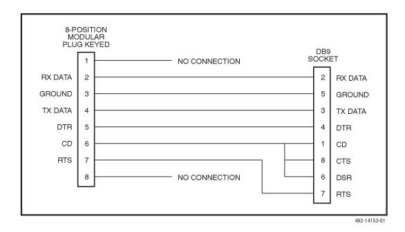
Figure D-5. COM Port-to-PC Cable
